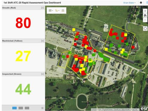
Results entered into the smartphone app were reported live to the operations center, using this color-coded display.
